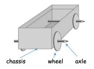
**Dowel** - wooden rod used for making the axles.
